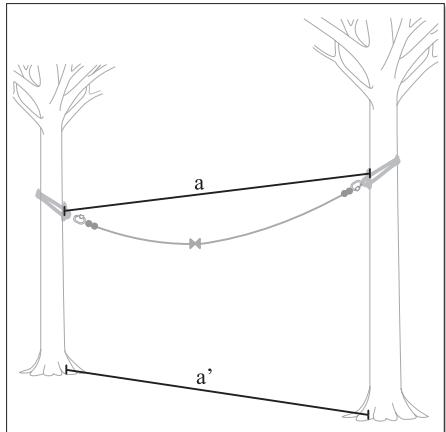
To determine the sag of a rope, the horizontal distance between the two suspension points (a) is measured. If, for example, both trees are quite straight, it is also possible to measure at ground level (a').
