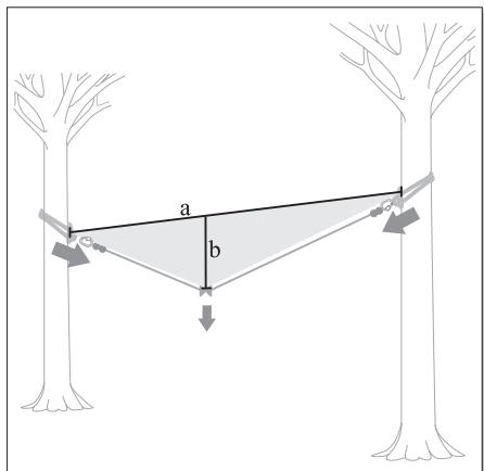
Then, measure or conservatively estimate the maximum distance that will occur between the loaded rope and the imagined horizontal line between the two suspension points (b). Divide the values (b divided by a) and you get the value of the sag. If the distance between the two trees (a) is 10 meters and the imagined horizontal line distance (b) is 2 meters, the value of the sag is 0.2 or 20%.
