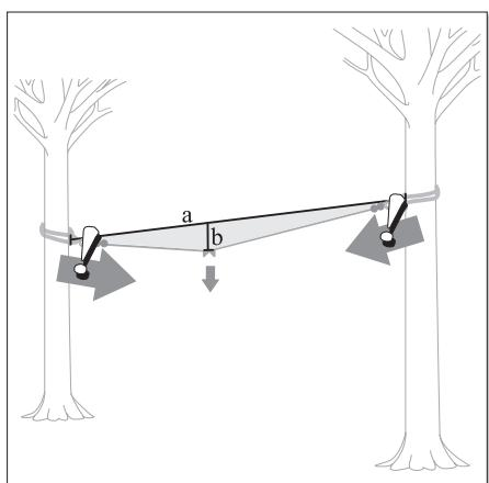
The following picture shows a smaller sag. The smaller the sag, the stronger the forces that affect the rope, the suspension points (carabiners), the heavy duty round slings, and the trees. This is shown in the following table.
